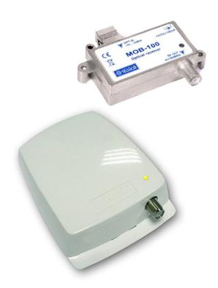
Micro optical receivers MOB-100 are the modern devices dedicated for FTTH (*Fiber To The Home*) applications. This device is made in die-cast metal housing and can be mounted in plastic housing "mouse" type. Receiver is equipped with SC/APC input connector and one RF output with "F" female connector. Optical receiver is also equipped with LED 3-stage optical input power indicator.
